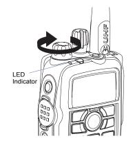
NOTE: The Home screen does not light up during a power up if the LED indicator is disabled (see *Turning the LED Indicator On or Off* on page 95).
