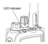
**NOTE:** The LED lights up solid green while the radio is transmitting and blinks green rapidly when the radio is receiving a privacy-enabled call.
