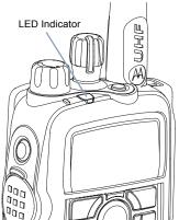
**Blinking red** – Radio is transmitting at low battery condition, receiving an emergency transmission or has failed the self-test upon powering up.
